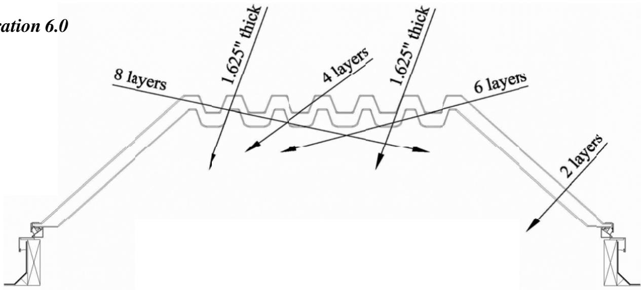
Light passing through the competing prismatic skylight highly complex, ribbed shape domes. Both the outer and inner domes have the same shape.
