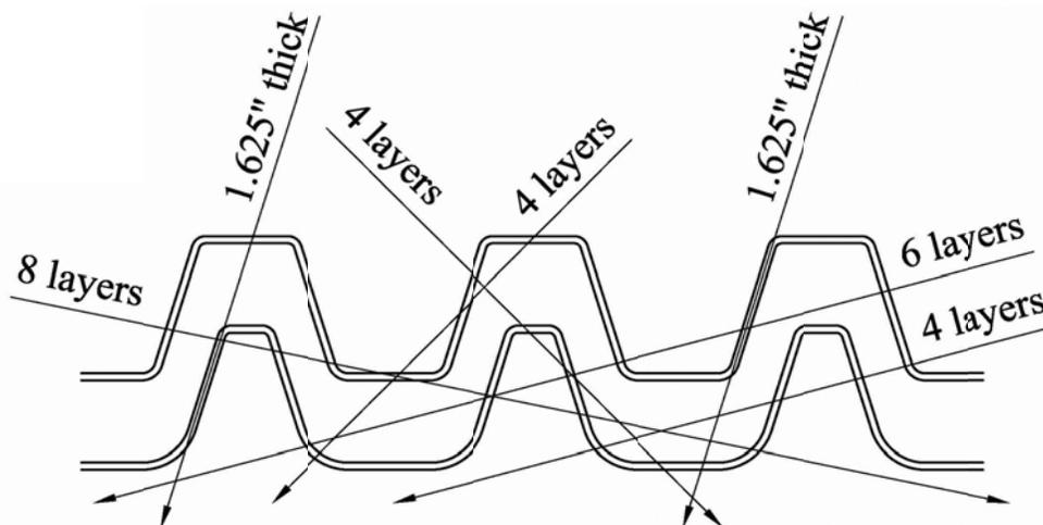
*A large portion of the available sunlight during the day must pass through multiple layers of the glazing and the twenty-four 1.625" long rib shoulders on the competing prismatic skylight unit.*
