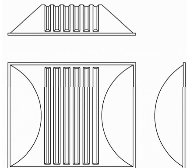
*Numerous ribs with steep shoulders and tight radii make this dome shape capable of utilizing thinner glazing but not without compromising light transmission.*
