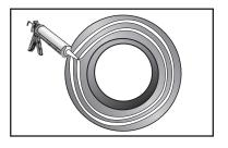
STEP 10 Taking care not to smear caulk on the exposed shingles, slide flashing under tar paper and shingles and force flashing up until the shingles come in contact with the raised portion of the flashing. The bottom side of the flashing will be on top of the shingles. Secure flashing with (6) Phillips head screws (D).
