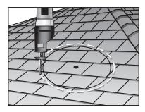
STEP 7 With a utility knife, cut a four inch slit through the shingles and tar paper at the 3:00 and 9:00 o'clock positions of the flashing. This allows for the footprint of the flashing to be inserted under the shingles.
