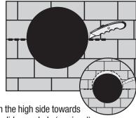
**NOTE:** Additional shingles may also need to be removed on the high side towards the ridge to allow the flashing to slide over hole (see inset).
