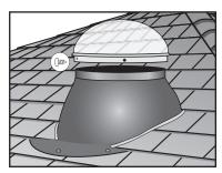
STEP 18 Remove paper backing from the adhesive tape on the U-channels (J) and place 1.5" from bottom of light pipe equidistant from each other so legs of the U-channels align vertically.
