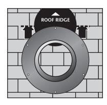
STEP 11 Apply caulk over all exposed screw heads (since they will be exposed to the weather). Use remaining caulk to seal the areas where the 4" slits were made and around area where shingles meet with raised area of the flashing.
