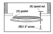
a dust free fit between the light pipe and the ceiling ring. Secure the ceiling ring to ceiling by inserting a 1 1/2" Phillips flathead screw **(M)** into one of the three pre-drilled dimpled holes and screwing it up through the drywall into speed nut **(K)** provided. Repeat this process for the other two screws.
