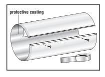
on both sides of seal to ensure a good bond. Secure the tube using the provided tek screws (I) - two screws per tube. Then place foil tape (F) over the entire seam to strengthen seal.
