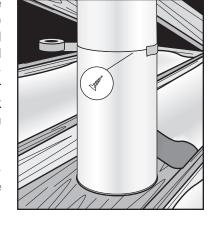
**IMPORTANT:** Remove protective coating that covers the mirror finish inside the tube.
