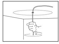
close to the desired installation area as possible. Mark the center of the ceiling ring **(L)**, drill a hole and insert piece of wire bent at a 90 degree angle. Rotate the wire around 360 degrees. While rotating, feel for resistance that could indicate wire runs or other obstructions.
