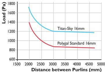
Wind Load vs. length of 16mm Titan Sheets at a constant deflection of 40mm, width 1050mm.
